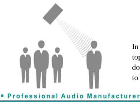
In case the directional speaker is mounted on the same wall – on top or below the digital sign, it needs to point diagonally downwards or upwards respectively, in order for the audio beam to reach all possible heights of users.
